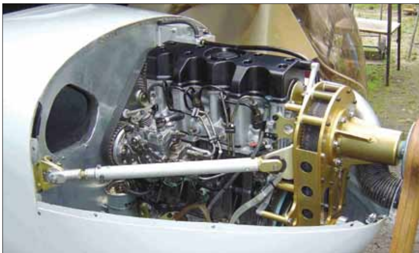
The PSA Peugeot 106 or Citroen AX engine. This is an aluminum-block engine, dropping weight to 176 pounds (80 kilograms) plus radiator and accessories. Pennec says the engine can be found for €300 in salvage form or €1,300 in exchange form.
