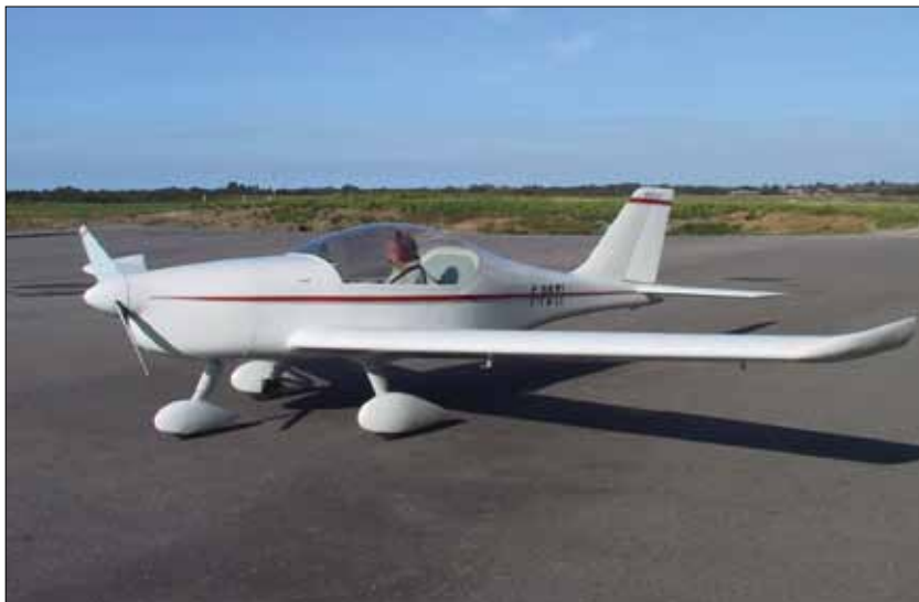
The prototype Dieselis with an Opel (identical to Isuzu equivalent) cast-iron engine. The airplane has well over 800 hours on it now with no difficulties.
