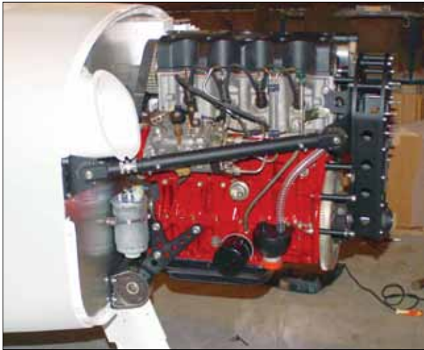
Gaz'aile can accept a range of diesel or gasoline-fueled engines. This is a PSA 1400cc unit.
