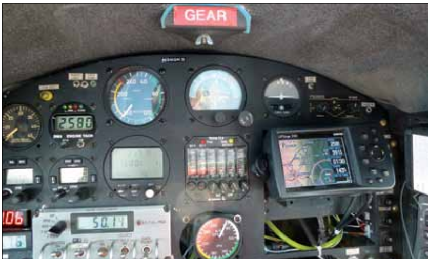
Panel of Klaus Savier's modified PV O-360 Lycoming-powered Long-EZ Determinator. "Cruising at 17,700 feet, 160 knots indicated, 217 knots true, 50 psi FP. The small airspeed reads a low amount of crank-case pressure. Fuel flow was about 8.2 gph. The gear warning is not recommended!...The Delaminator has the more efficient O-200 from the Cessna 150s. It cruises at the same 17,500 feet at about 195 KTAS and 4.2 gph," Savier said.
