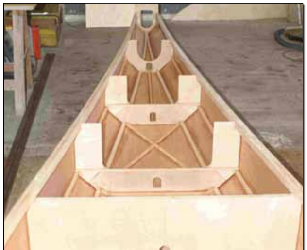
The Gaz'aile's fuselage is almost all wood. The wings are wood, foam and carbon fiber.
