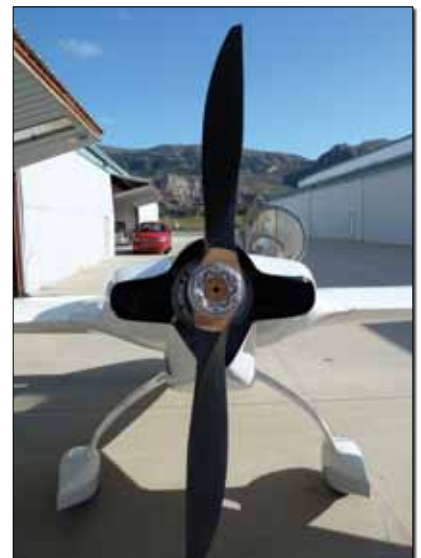
Delaminator's 67-inch-diameter, 101-inch-pitch propeller—one element in high-mpg performance.
