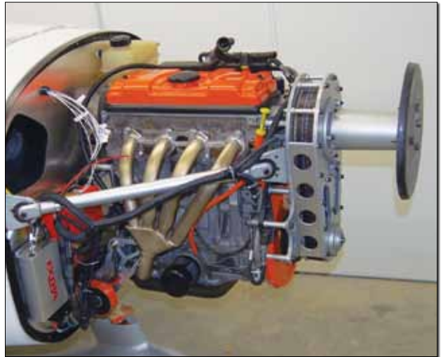
The gasoline engine works well in Gaz'aile, too, giving 124-mph cruise and burning only 3.44 gallons (9.2 liters) per hour, giving 36 mpg.
