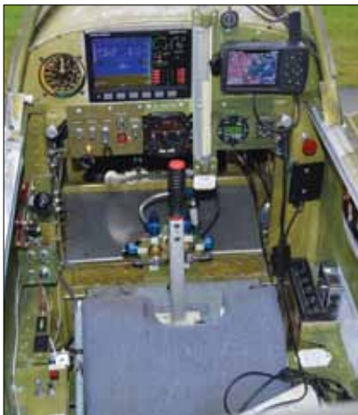
The E-1 cockpit reflects Ebnetter's 20,200 hours of experience and military background. Note the open and readable fuel-transfer selector. (Photo: Arnold Ebnetter)
