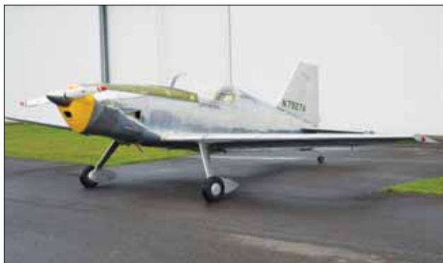
The E-1 as configured for record efficiency flight, with Sensenich ground-adjustable prop, a new spinner and a mixture control, as well as simple wheel fairings. (Photo: Arnold Ebneter)
